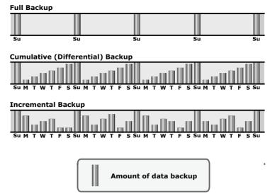
Figure 12-1: Backup granularity levels
