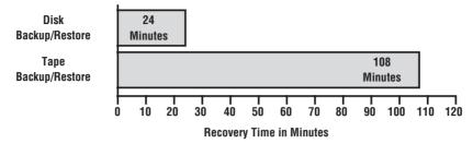
Figure 12-17: Tape versus disk restore
