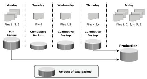
Figure 12-3: Restoring a cumulative backup
