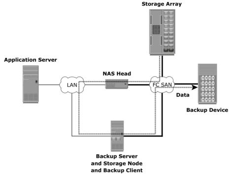
Figure 12-12: Serverless backup in NAS environment
