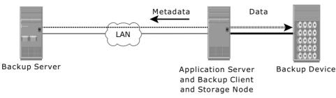
Figure 12-7: Direct-attached backup topology
