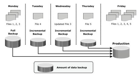
Figure 12-2: Restoring from an incremental backup
