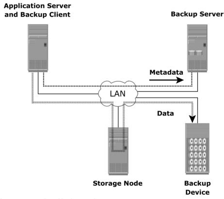
Figure 12-8: LAN-based backup topology
