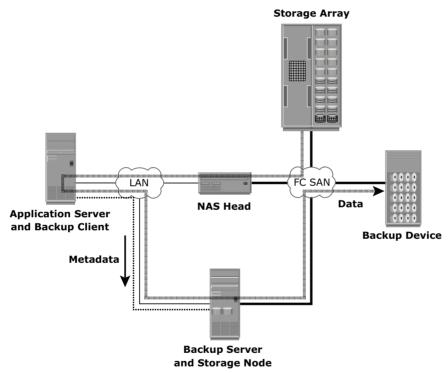
Figure 12-11: Server-based backup in NAS environment
