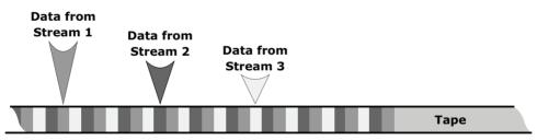
Figure 12-16: Multiple streams on tape media
